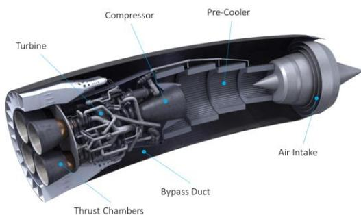
Figure 2: SABRE 3 (Reaction Engines)
