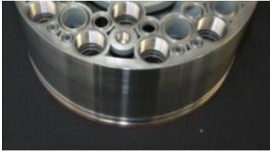
*Figure 4: 3D printed injector system for the Advanced Nozzle Project*
