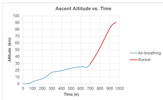
Figure 7: Skylon Standard Mission Ascent Altitude Vs. Time (Reaction Engines)
